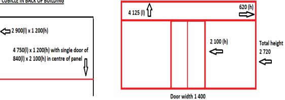
ALUMINIUM FRAME WITH DOUBLE DOOR TO REPLACE OFFICE WALL
