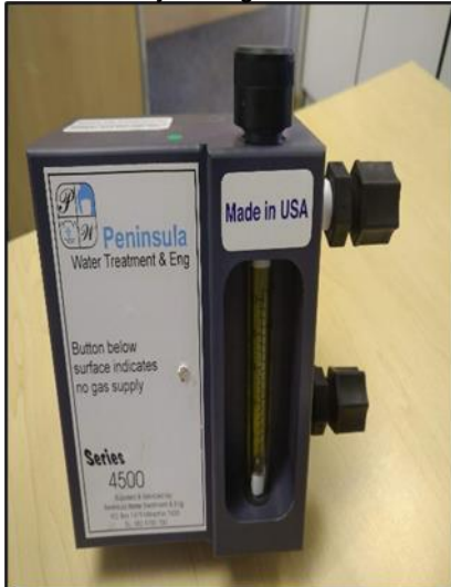
Sample of mounted gas chlorinator
